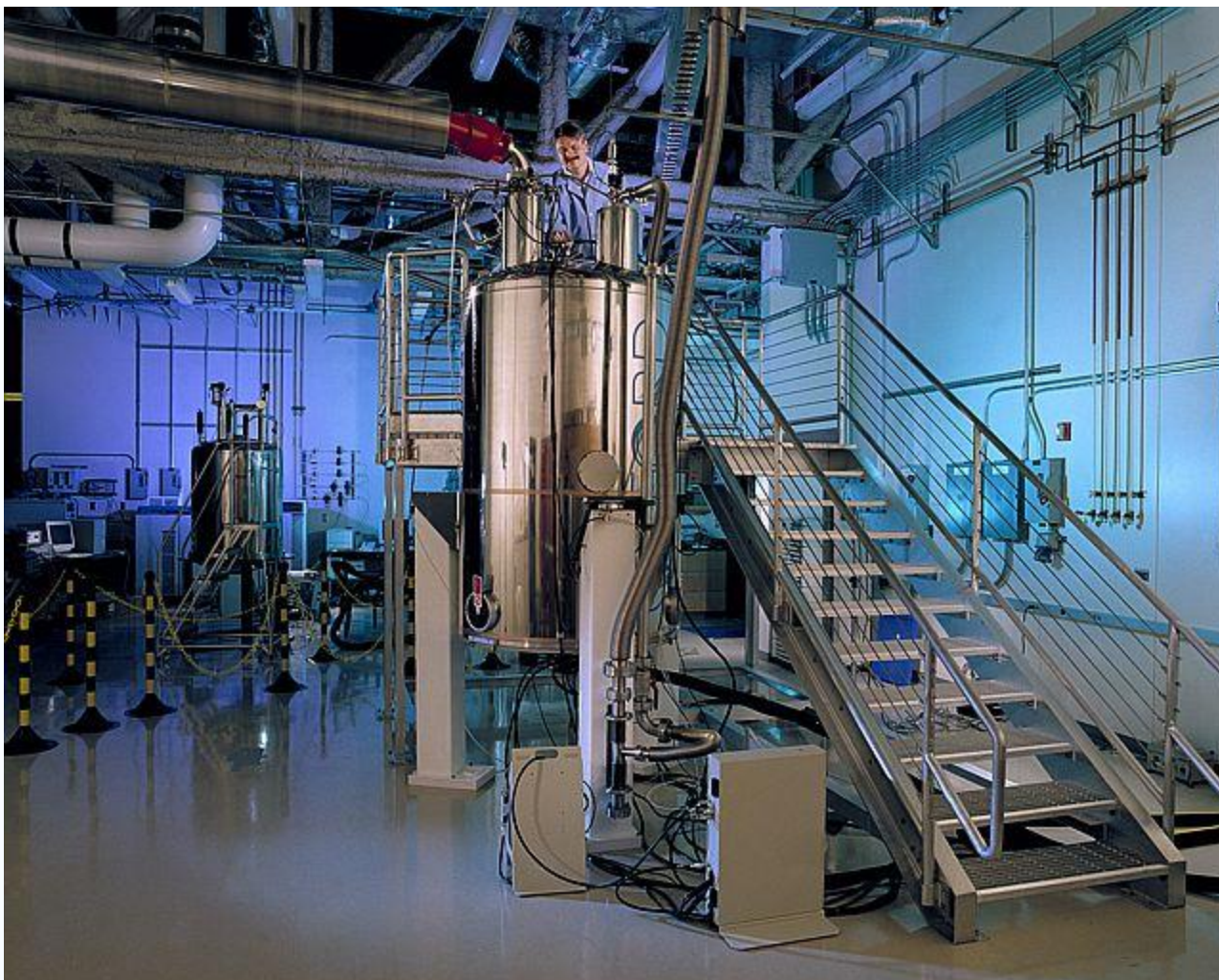
Northwest National Lab – 800 MHz NMR – note superconducting magnet dewar
