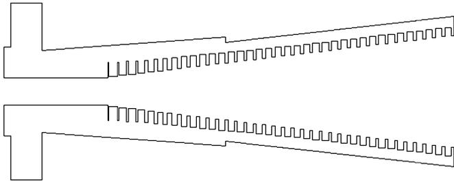
Fig. 2. Cross section of electroformed horn.
