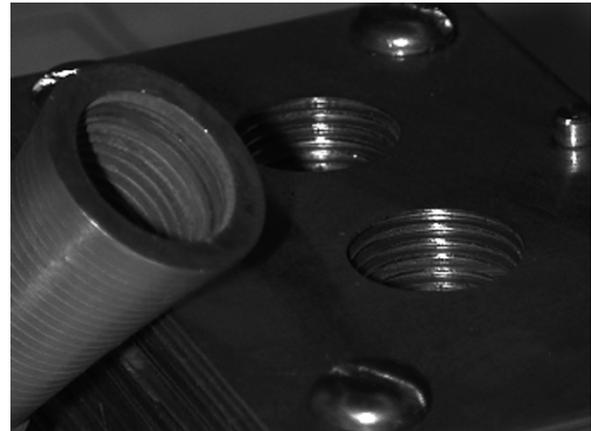
Fig. 1. 100-GHz platelet and electroformed horns.
