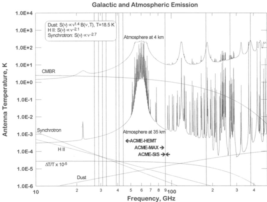
**FIGURE 1.** Atmospheric emission and representative galactic foregrounds are shown compared to the expected level of anisotropy. The atmosphere at 4 km is relevant to observations made from the South Pole while the atmosphere at 35 km is relevant to balloon borne anisotropy measurements. The vertical lines represent the band centers of the various receivers which have been used on the ACME platform.
