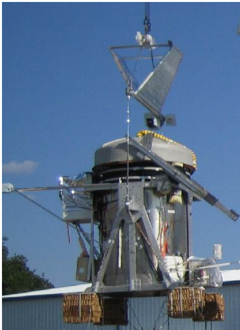
FIG. 5.— Photograph of the ARCADE 2 instrument just prior to 2006 flight. The instrument core is contained within the large (1.5 m diameter, 2.4 m tall) bucket dewar. The lid is shown closed for launch. The electronics box containing the warm stages of the radiometers and the payload electronics is mounted to the left of the dewar, and the three-axis magnetometers to determine orientation relative to the Earth's magnetic field are seen to the left of the electronics box at the edge of the frame. The reflector plate is visible at the top of the photo above the lid. Cardboard pads at the four bottom corners absorb some of the impact when the payload hits the ground upon termination of the flight.
