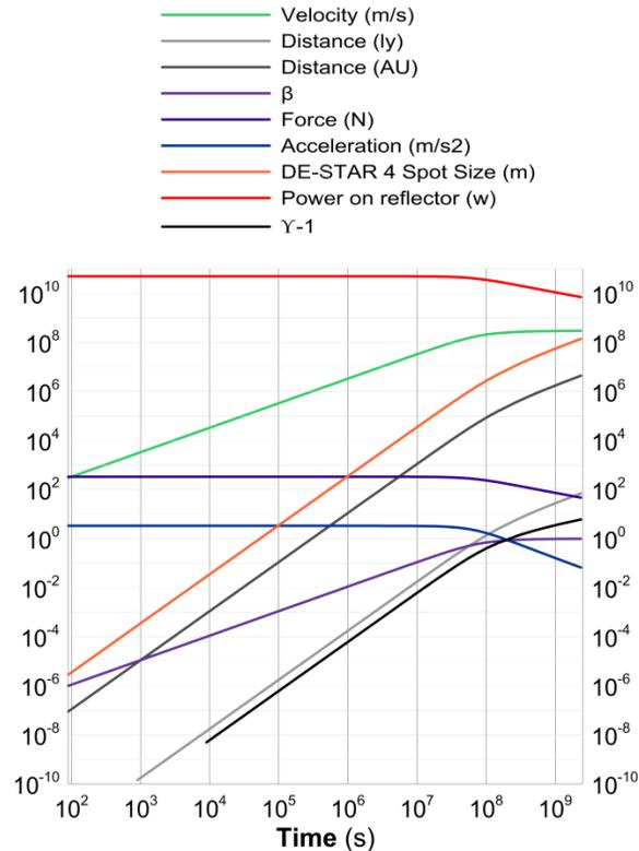
**Figure 8.** Numerical solution to relativistic equation of motion for 100 kg rest mass with a reflector that is assumed to grow as large as is needed to intercept the full beam and a DE-STAR 4 - 50 GW drive. As discussed the case of a fixed reflector of 30 m diameter that is reasonable for a 100 kg craft will only reach about 3% the speed of light and then coast. The decrease of power on the reflector is from relativistic effects.
