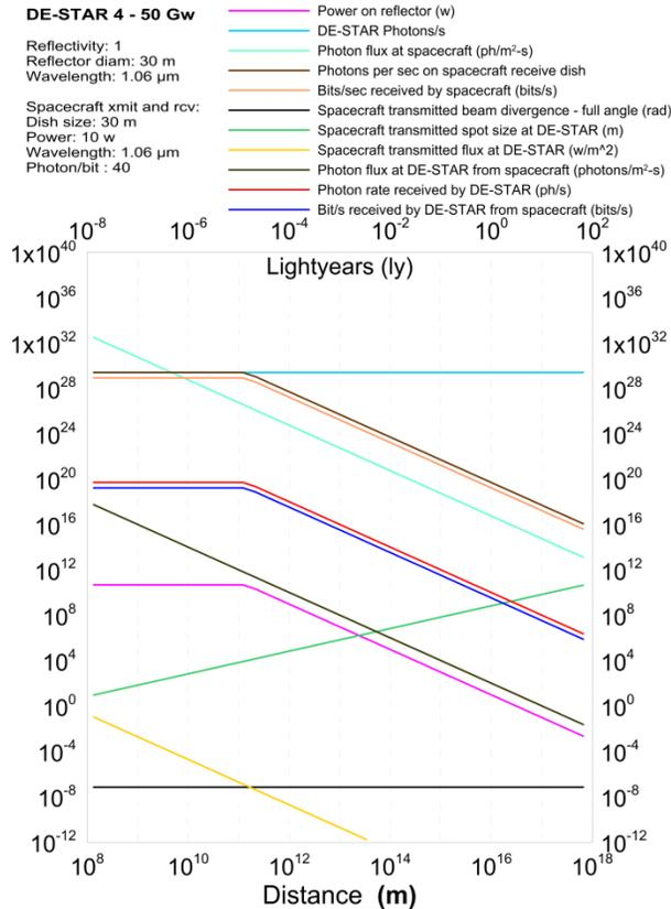
**Figure 10.** Communications parameters between a DE-STAR 4 and a small robotic spacecraft vs. distance to spacecraft. The spacecraft is assumed to have a 10 watt burst mode (hibernates most of the time) IR transmitter and uses a 30 m reflector as both the drive and the transmit/receive reflector. Both uplink (DE-STAR to spacecraft) and downlink (spacecraft to DE-STAR) are shown.
