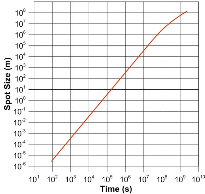
**Figure 5.** Plot of DE-STAR spot size (reflector size required) with respect to time for the 100 kg craft case. This assumes the reflector is illuminated fully the entire time.
