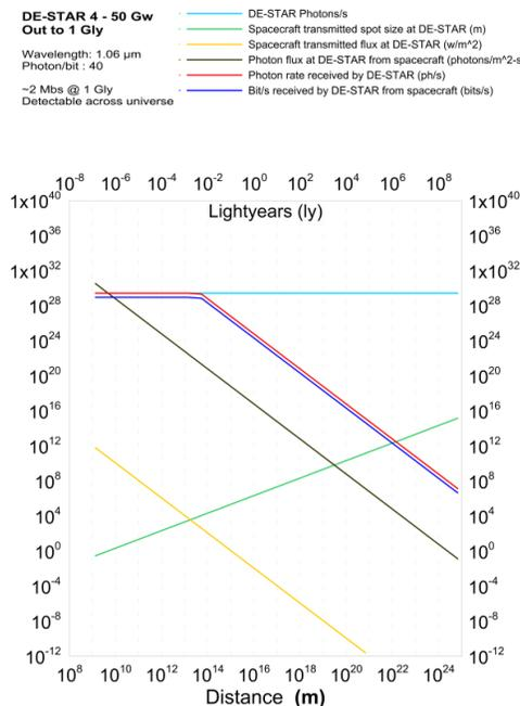
**Figure 11.** Communications or searches between two civilizations with DE-STAR 4 units at each civilization vs distance out to 1 Gly. The conclusion is that we would get an equivalent bit rate at 1 Gly of about 2 Mbps. This implies that this "modest" technology that we have now advanced to envisioning implies that civilizations across the entire universe could send high speed information to each other modulo the time of flight. The implications for SETI searches are profound.
