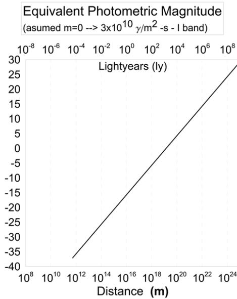
**Figure 12.** Photometric (broad band equivalent) magnitude vs distance for a DE-STAR 4 out to 1 Gly. The I band equivalent photometric magnitude at 1 Gly form a DE-STAR 4 is approximate  $m = 30$  or roughly the limit of the HST.
