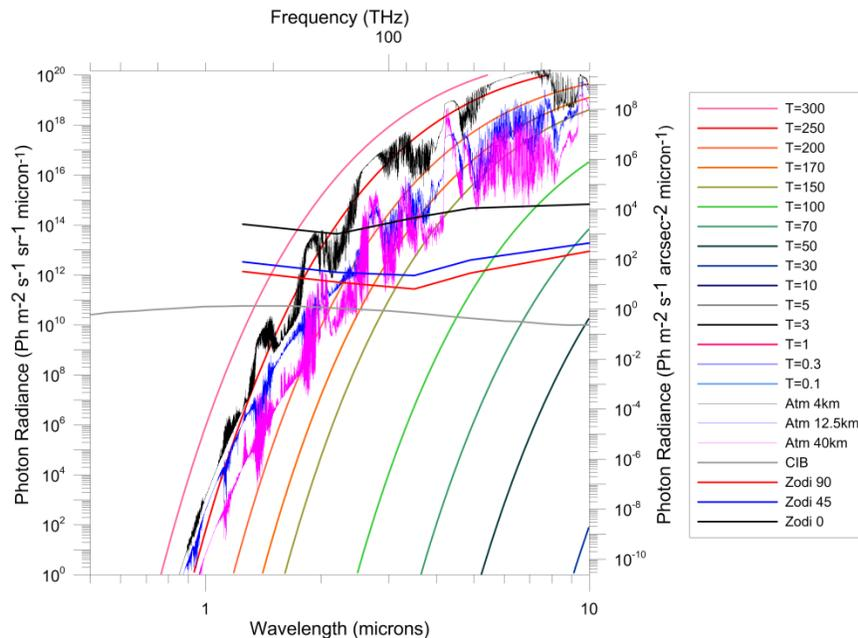
**Figure 15.** Comparison of optical emission vs optics temperature assuming emissivity is unity, atmospheric emission for various altitudes, Cosmic Infrared Background and Zodiacal light at various ecliptic inclinations (day 100 from COBE) vs wavelength for  $0.5$  to  $10 \mu\text{m}$ . Note the left hand and right hand vertical axes are reversed compared to Figure 13 and 14. The bottom line is that at  $1 \mu\text{m}$ ; the optical emission is small compared to the Zodi and CIB.
