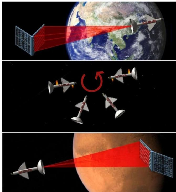
**Figure 16.** A second DE-STAR photon drive at the mission destination can decelerated the spacecraft under controlled conditions. This deceleration is achieved by a "ping-pong" method where the spacecraft rotates and first one DE-STAR and then the second provide opposing forces to the reflector.
