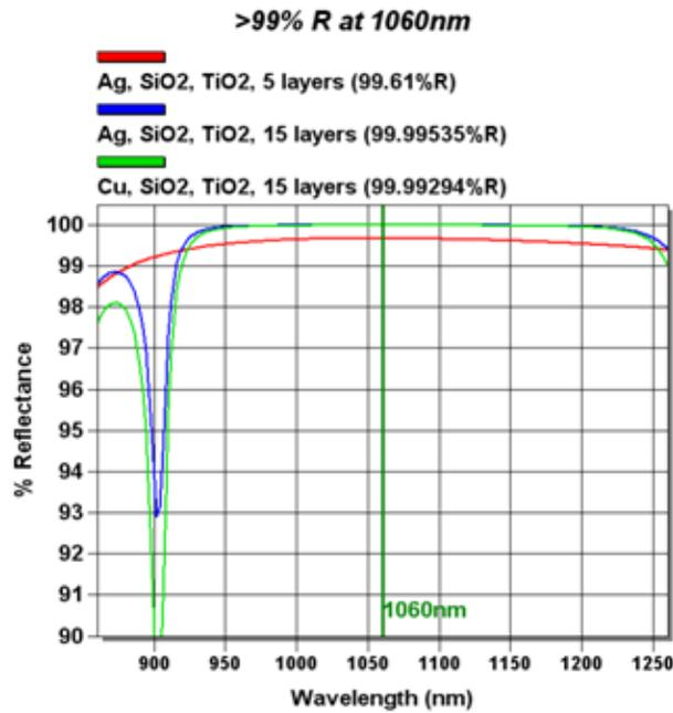
**Figure 9.** Graph of the percent reflectance for a practical thin film roll to roll reflector design. The green line of 1,060 nm corresponds to DE-STAR's laser wavelength. (Source: figure and data from Surface Optics - private communications (2013)). Reflectivities in excess of 99.995% are achievable now on thin film plastics and with further refinements 99.999% looks feasible.
