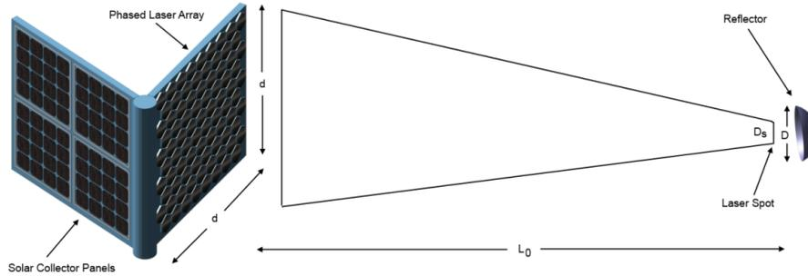
**Figure 2.** Diagram depicting relevant variables.  $L$  is the distance to the spacecraft and  $L_0$  denotes the distance of the spacecraft when the beam spot equals the reflector size. As the spacecraft moves outward, the laser spot size ( $D_s$ ) increases in proportion to the distance  $L$  to the spacecraft and ultimately,  $D_s$  becomes larger than  $D$  at which point the photon force begins to decrease proportional to the ratio of the spot to reflector area or  $(D_s/D)^2$ .
