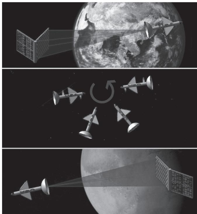
**Fig. 16** A second DE-STAR photon drive at the mission destination can decelerated the spacecraft under controlled conditions. This deceleration is achieved by a “ping-pong” method where the spacecraft rotates and first one DE-STAR and then the second provide opposing forces to the reflector.
