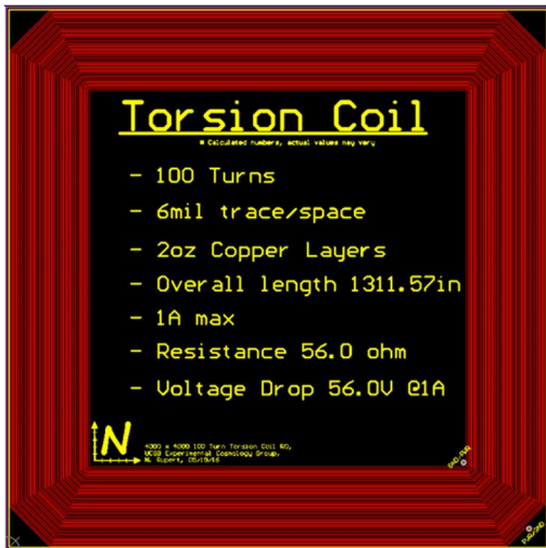
Figure 2. Computer generated image of the torsion coils used for alignment of LEO WaferSat.
