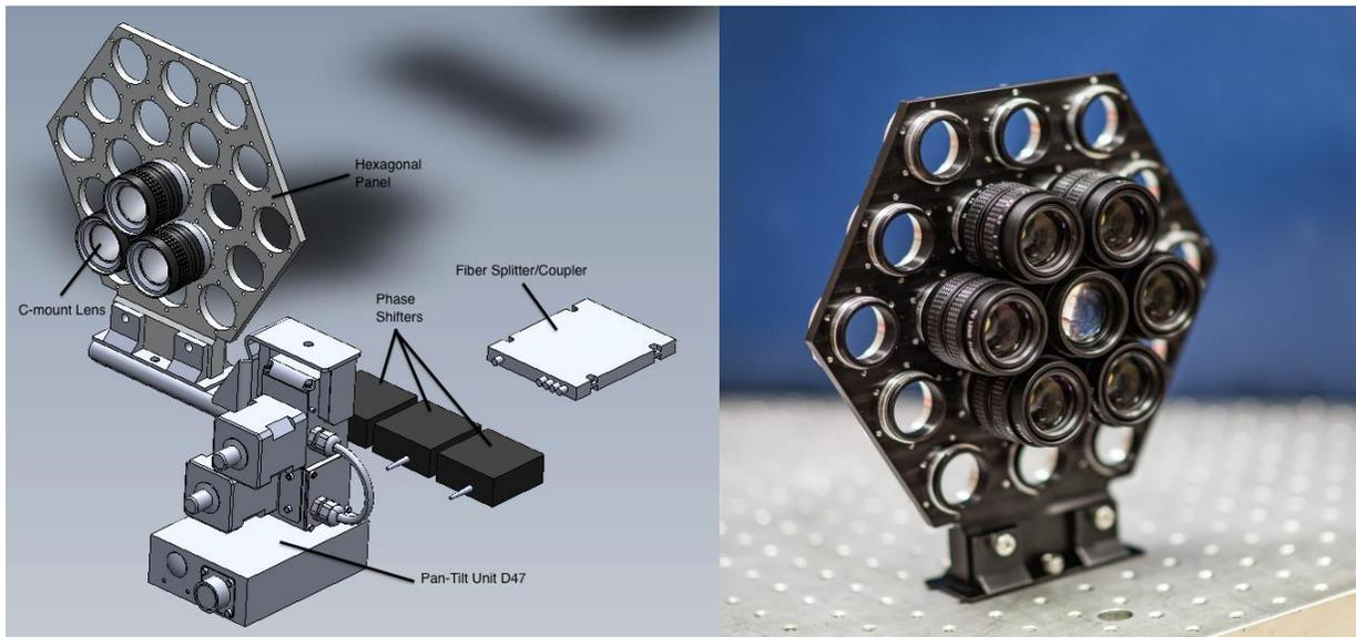
**Figures 2 and 3:** CAD rendering and photo of the quarter-scale model, including lenses mounted in an aluminum panel.
