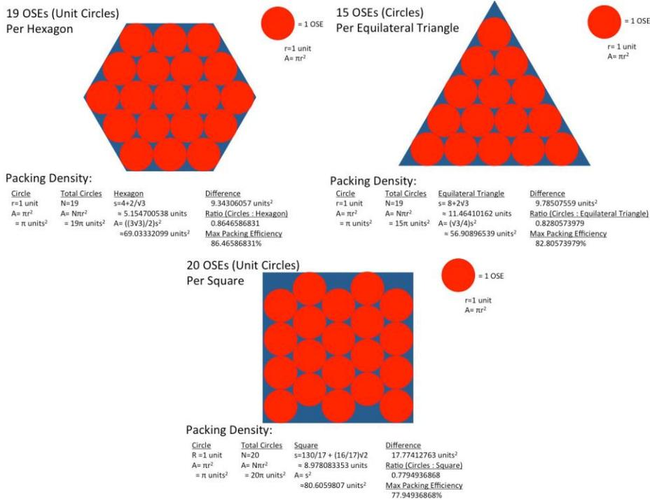
**Figure 5:** Triangular, Hexagonal, and Square BOA with Maximum OSEs
