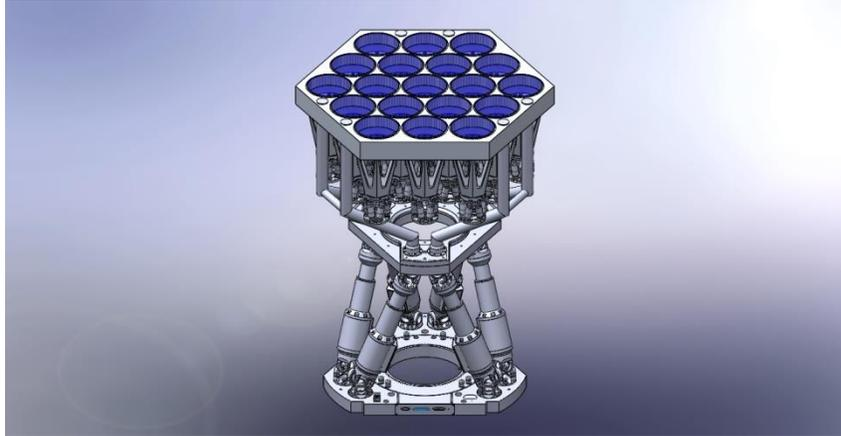
**Figure 1:** CAD rendering of a square-meter telescope; LAST will contain over one million of these sub-arrays.
