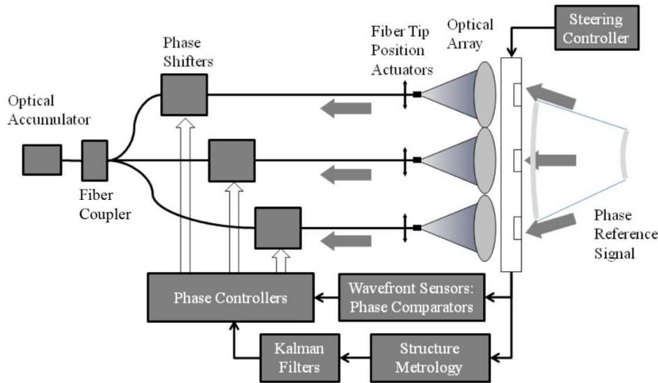
Figure 4: Annotated schematic of the optical assembly
